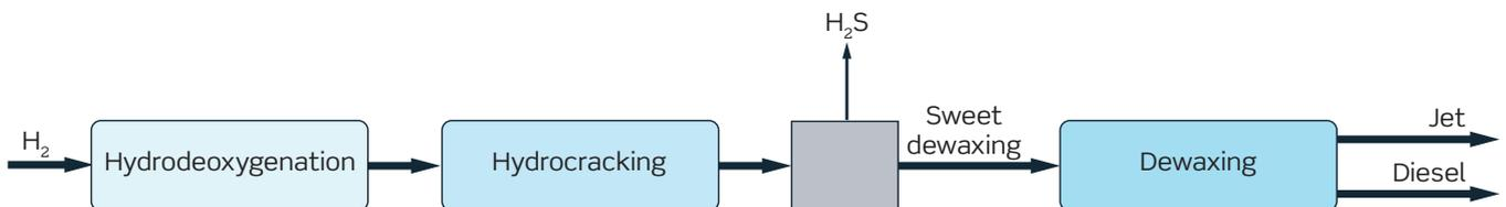
Figure 4. Simplified flow sheet of sweet mode HydroFlex™.
