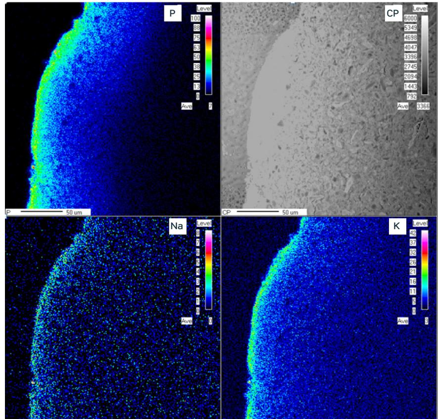
Figure 1. SEM picture of a high phosphorus-containing crust around a guard catalyst from a commercial unit processing 50% renewable feedstock.
